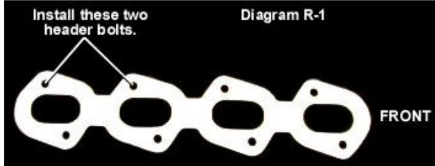
**NOTE:** Some header flange bolt holes are slotted for the ease of bolt installation and are not intended to be installed before the header is inserted into the engine bay. Only the bolts specified in the installation procedure should be installed before the header is inserted into the engine bay.
