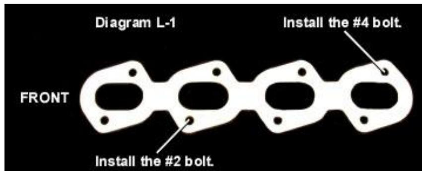
**NOTE:** Some header flange bolt holes are slotted for the ease of bolt installation and are not intended to be installed before the header is inserted into the engine bay. Only the bolts specified in the installation procedure should be installed before the header is inserted into the engine bay.
