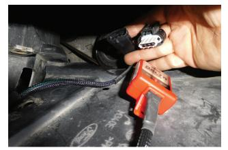
6. Connect male connector on Delta Boost module into factory sensor. Connect female connector on Delta Boost module with connector on factory harness.
