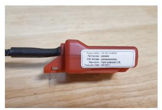
2. Record MAC address on side of your Delta Boost module. It will be necessary later to establish a connection with Delta Boost smart phone app.
