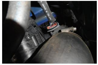
5. Unplug sensor by squeezing locking tab at its top and pulling plug.
