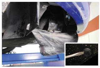
4. Remove clips then carefully pry inner fender well back enough to expose driver side of intercooler and locate boost sensor.
