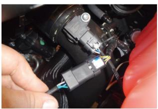
Connect male connector on module to factory sensor. Connect female on module to connector on factory harness. Set module on right side.
