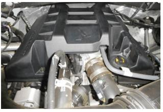
The pressure sensor is located at front of engine. Disconnect wiring harness from pressure sensor.
