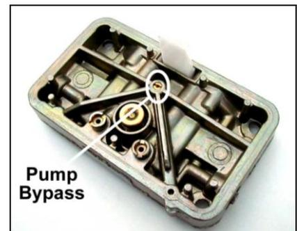
**NOTE:** The emulsion bleed tuning kit (P/N 36-322) is designed to support the tuning efforts of this new block. It contains ten each of the following bleed sizes: Blank (no hole), .020”, .031”, .040”, .046”, and .052”. Individual bleeds are available from blanks to .078” from your Holley dealer under individual P/Ns 142-xx (xx=size).
