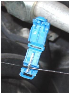
**Figure 4 (T-Tap connector installation)**
