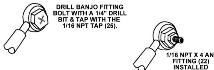
Figure 8 Schematic of "Drilled Out" Banjo Fitting
