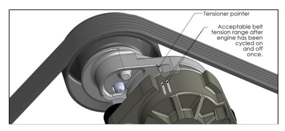
**NOTE:** If you are NOT using all the Holley accessories supplied, or have changed the original crank or any accessory's pulleys, you will have to measure to find the correct belt length.
