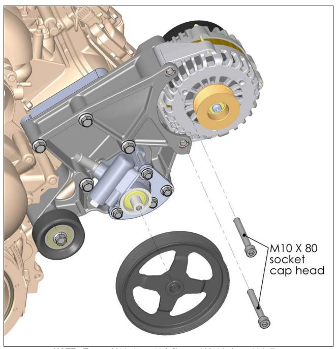
**NOTE:** Torque M8 bolts to 18 ft./lbs. and M10 bolts to 36 ft./lbs.
