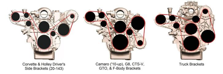
**HELPFUL HINT:** When installing the belt, route around all the pulleys except the water pump pulley. While fully rotating the tensioner arm, slip the belt on the smooth water pump pulley last.
