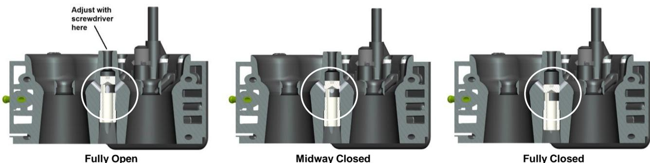
The idle bypass valve allows for additional airflow through the carburetor, while maintaining the desired relationship between the throttle plate and the transfer slot. Applications using a larger cam may benefit most from this new feature. This valve replaces the need for holes in the throttle plates.
