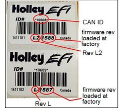
The Rev L2 and newer ECUs have updates to the thermistor inputs (coolant and air temperature sensors) for increased accuracy at low temperatures when using Ford sensors. Earlier ECUs have less than ideal temperature sensor accuracy under cold ambient conditions (less than about 50° F) when using Ford sensors.
