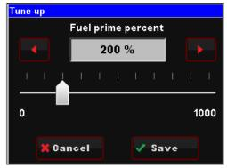
**NOTE:** This only injects fuel once at key-on, and will not do it again until the engine has run. This fuel prime occurs ½ of a second after key-on. If you quickly turn the ignition key without waiting for ½ a second, the prime will not occur and it may take longer for the engine to start.
