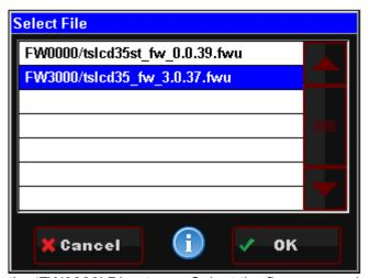
V3 Firmware is preloaded in the 'FW3000' Directory – Select the firmware and select 'OK' to update the 3.5
