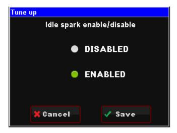
NOTE: This feature should be disabled when checking base timing with a timing light!
