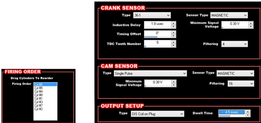
There are calibrations built into the Holley software for many of the common factory sensors, but they need to be selected as well. These built in calibrations cover most of the Ford Modular applications and can be selected in the Sensors ICF:
