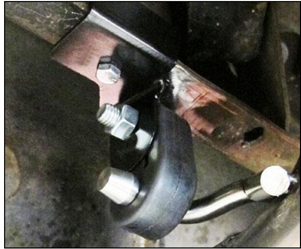
Figure 4 – Right tailpipe hanger bracket
