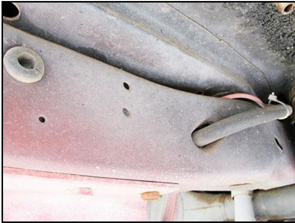
Figure 5 – Right side frame attachment holes
