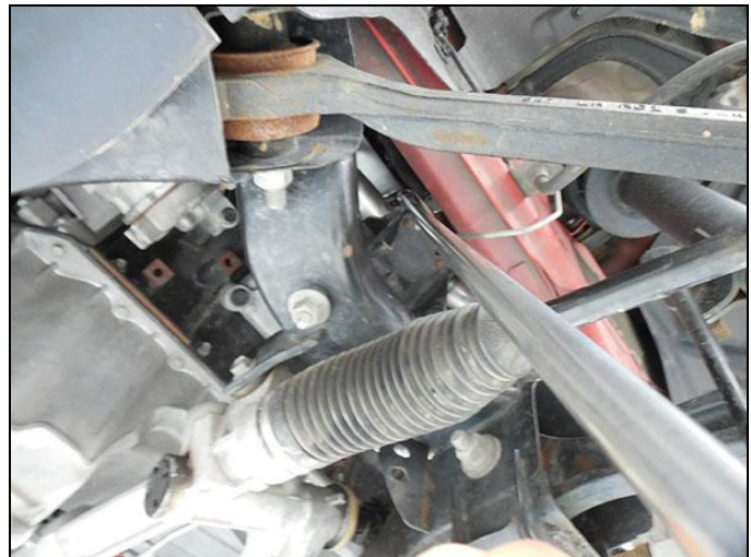
Figure 2 – Access to top bolts - driver's side
