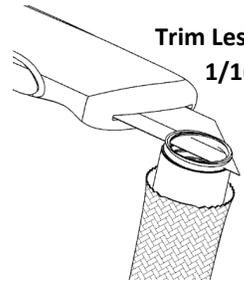
**4** Trim the hose to be flush and square with the olive using a sharp blade. **Trim Less Than 1/16"**
