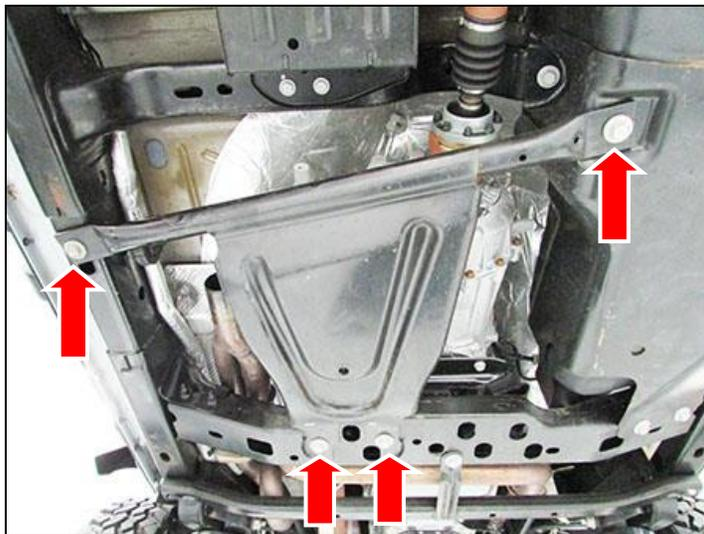
5. Remove the muffler and mid pipe exhaust.
