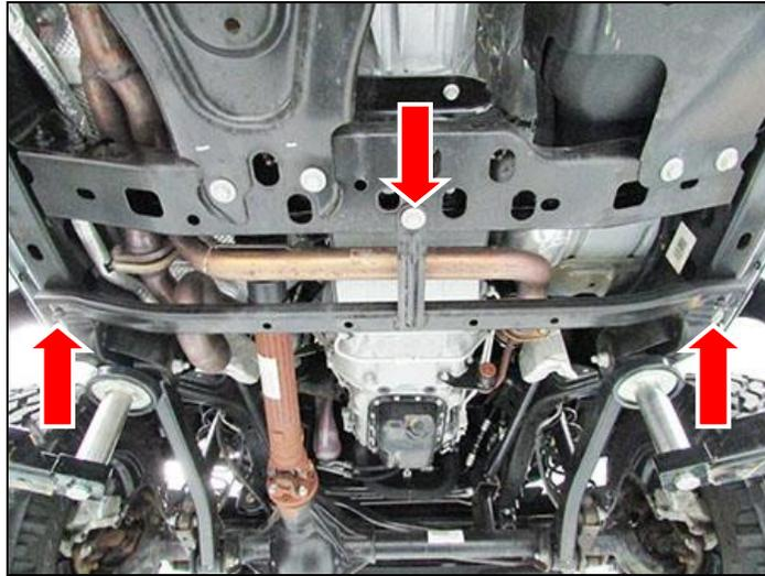
4. Remove the skid plate behind the lower cross member.
