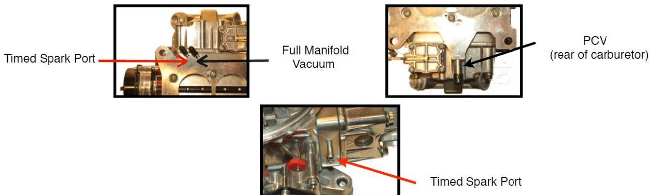
Distributor vacuum advance may also be connected to the tube in the primary metering block.
