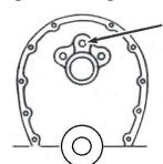
CAUTION: When installing the center oil galley plug on a small block Chevy, do not tap this plug in too deep or you will block the oil passage to the front cam bearing.
