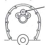
CAUTION: When installing the center oil galley plug on a small block Chevy, do not tap this plug in too deep or you will block the oil passage to the front cam bearing.
