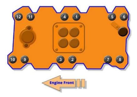
7. On the underside of the intake manifold plenum area, there is a flange with (x4) holes tapped. (x1) 1/4" NPT and (x3) 3/8" NPT fittings are provided. These ports will provide ample vacuum port sources for your manifold. Any of these ports can be utilized depending on required needs. Any unused ports can be easily plugged or an NPT fitting can be capped for later use as needed.
