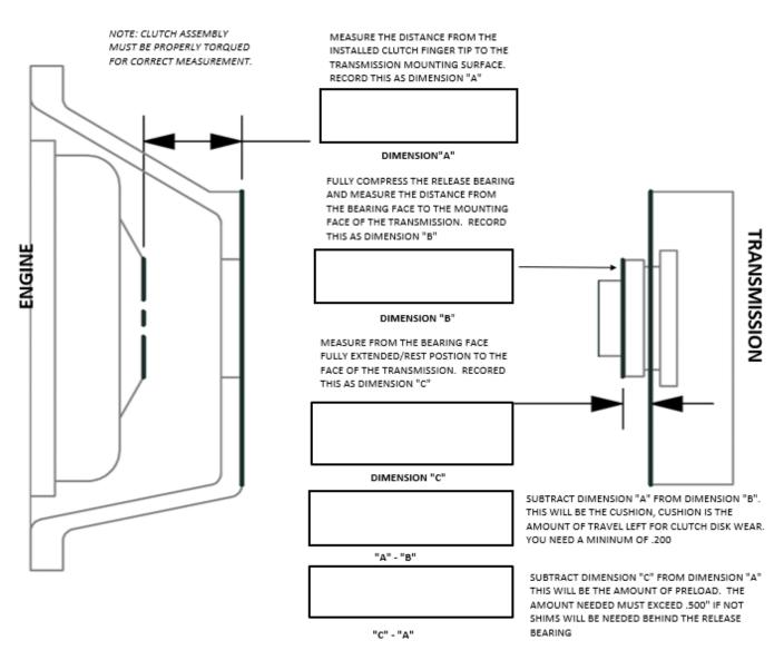
NOTE: All fasteners for the engine side or transmission side should be torqued between 35 and 45 ft./lbs. to maintain parallelism. It is more important that they are all torqued the same more than whether it is 35 or 45 ft /lbs.
