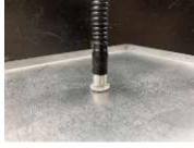
10. Remove bolt and washer & replace with ORB Plug. Install adapter of your choice (sold separately) at front of fitting as shown. Connect return line and check for leaks.
