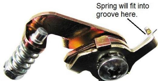
Spring will fit into groove here.
