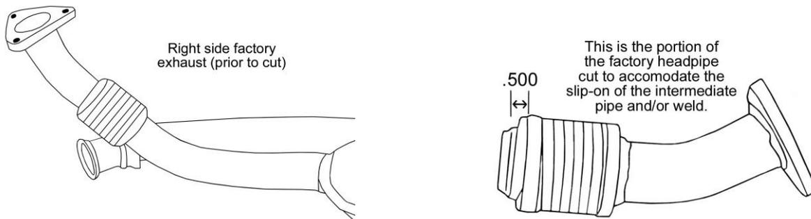
9. Attach the intermediate exhaust pipe (supplied with header) to the header, leaving it loose to rotate.
