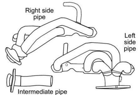
**WARNING! Breaking in an engine with ceramic-coated headers WILL result in damage to the coating and will VOID all warranties. Ceramic-coated headers require several heat cycles to fully cure before they will withstand extreme heat. HOOKER recommends using a cast-iron exhaust manifold or an old header to break in new engines to avoid coating damage.**
