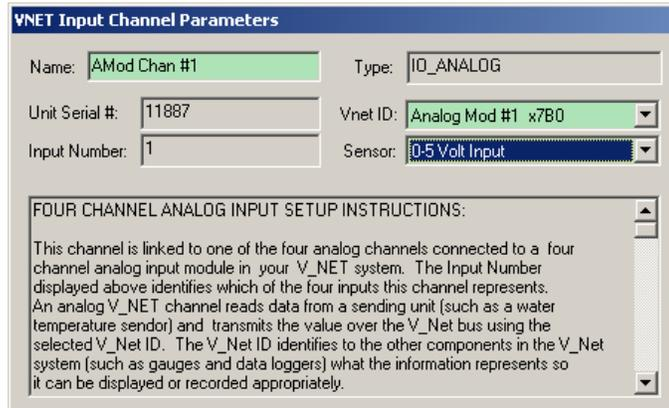
Locate the **Four Channel Analog Input Setup Instruction** text box. This text box provides online instructions for modifying the setup of this module. Read the instructions and modify the setup as desired. (Please note the scroll bar located on the left-hand portion of the text box is used to scroll through the instructions).
