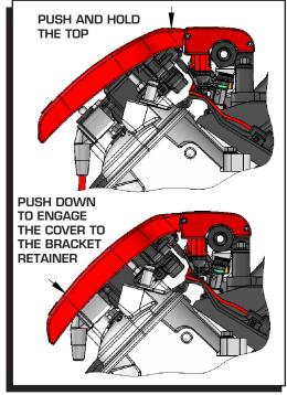
Figure 7 Installing the Coil Covers.
