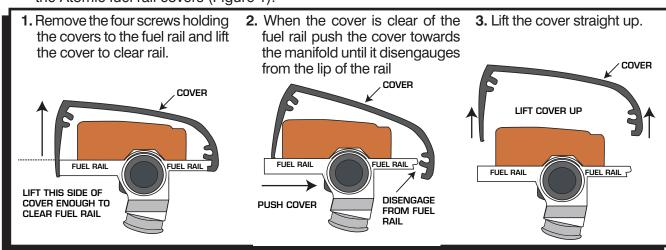
Figure 1 Removing the Fuel Rail Covers.
