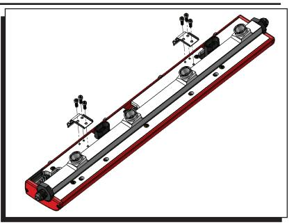
Figure 2 Coil Cover Bracket Installation.
