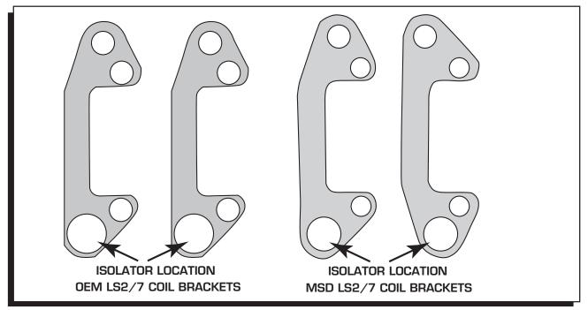
Figure 3 Installing the Isolators.
