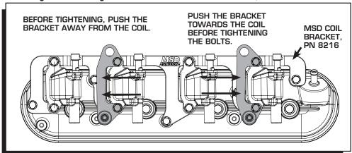
Figure 5 Installing the Coil Cover Brackets with MSD's LS2/7 Aluminum Coil Brackets.
