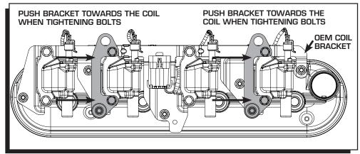
Figure 4 Installing the Coil Cover Brackets with OEM LS2/7 Coil Brackets.
