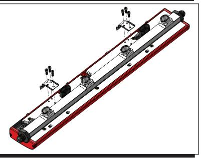
Figure 2 Coil Cover Bracket Installation.
