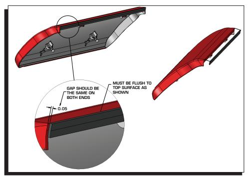
Figure 6 Applying Foam Tape to Unfinished Covers.
