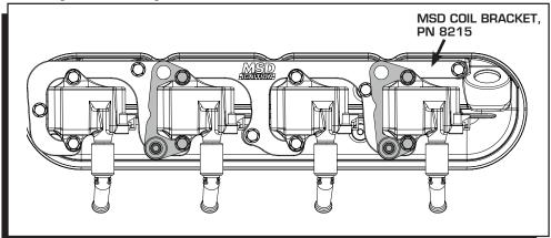
Figure 5 Installing the Coil Cover Brackets with MSD's LS1/6 Aluminum Coil Brackets.
