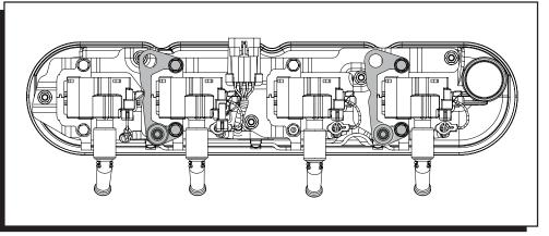
Figure 4 Installing the Coil Cover Brackets with OEM LS1/6 Coil Brackets.
