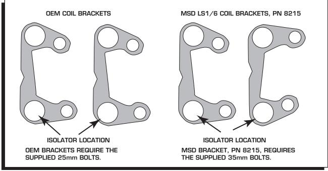
Figure 3 Installing the Isolators.
