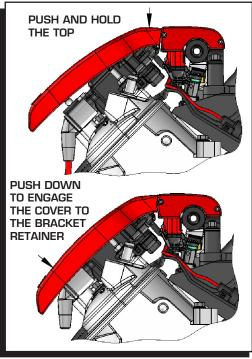
Figure 7 Installing the Coil Covers.
