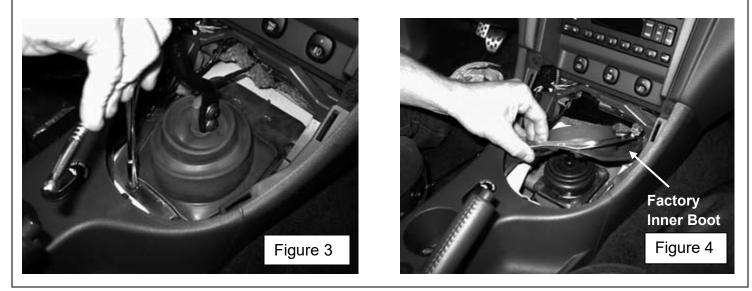
5. Using a 13mm socket, remove four (4) hex head bolts that fasten stock shifter assembly to transmission. Discard bolts, new ones are supplied. Lift shifter assembly straight up and off. **NOTE:** You may have some difficulty in removing stock shifter from transmission due to adhesive sealant applied at factory.
