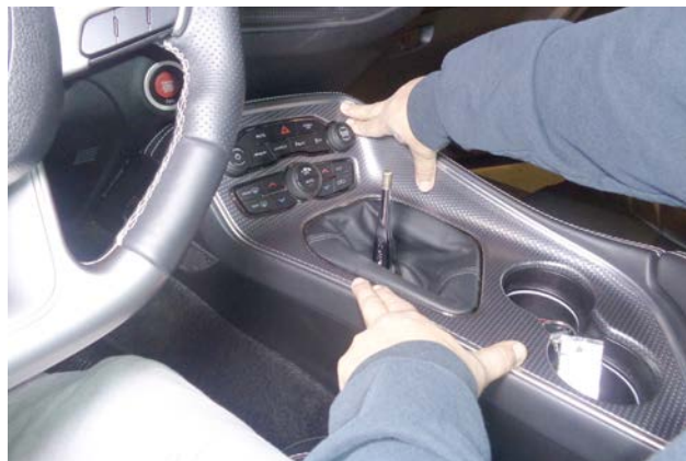
70. Snap the console bezel into the console.
