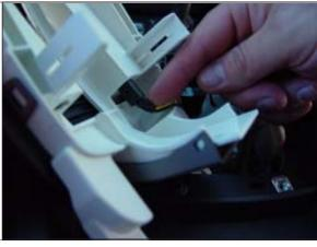
**STEP 11.** Carefully, unsnap the tabs of the shifter cover plate to remove it from the white plastic shifter frame.
