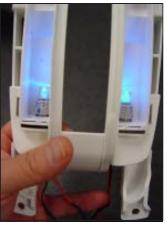
**STEP 19.** Place the black plastic slider into the track of the white plastic frame with the original red indicator on the driver's side of the vehicle (the newly installed indicator on the passenger side). Then snap the Hurst plate onto the white plastic frame making sure the cut-outs on the plate engage the tabs on the white plastic frame on all four (4) ears.
