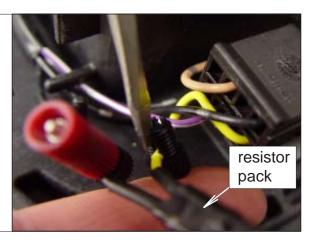
**STEP 17.** Unscrew each wire tap head (red end with hole) off of each wire tap body. Feed each black wire end (2) from the ABL LEDs through one of the wire tap head holes and screw it onto the wire tap body that is connected to the black wire. Feed each (2) red wire end from the ABL LEDs through the other wire tap head hole and screw it onto the wire tap body that is connected to the yellow wire.
