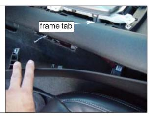
**STEP 9.** From under the center console access the white plastic shifter cover frame tabs on both sides and lightly pull the tabs outward to release the frame from the shifter assembly.
