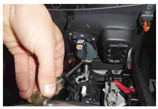
Remove factory set screw located at base of shift handle. Pull straight up on shift handle to remove handle and bezel assembly.
