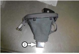
18. Slide boot up pistol grip base as far as it will go. Then apply a small drop of thread locking fluid to set screw (2) threads and start it in pistol grip.
