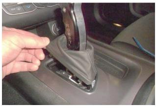
21. Clip shifter boot back into bezel. Shift through all positions to ensure proper installation.
