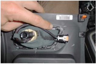
6. Release clips (x4) to remove shift boot and factory handle from bezel.
