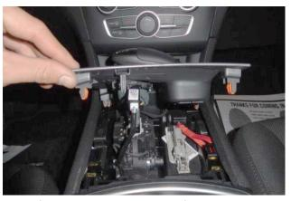
4. Lift up on bezel then unplug shift handle harness connector.
