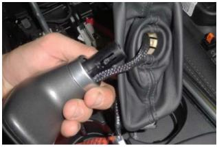
Separate shift boot from shift handle and wire harness.
