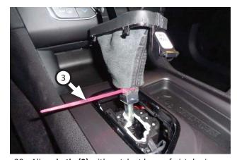
20. Align **zip tie (3)** with notch at base of pistol grip. Tighten zip tie and trim excess.
