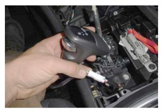
13. The factory shifter features a computer chip for illuminated gear select indicator. If disconnected, the vehicle ECM will not see it and an error light will be generated. To remedy this, plug factory shift handle back into factory connector.
