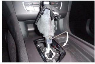
19. Slide pistol grip about halfway down shift rod. Run set screw in until it bears lightly on shift rod. This assists in aligning set screw with dimple on shift rod. After it is aligned, tighten screw fully.
