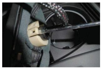
8. Release clips (x2) that mount shift boot retaining collar to shift handle.
