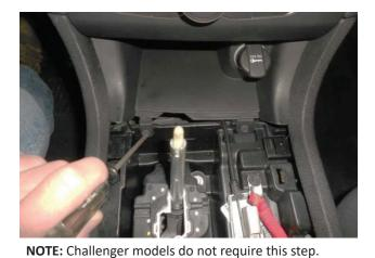
Remove screws (x2) from front console storage tray.
