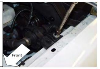
7. Remove portion of OEM Induction Tube going through the driver's side firewall. Lift Induction Tube above Master Cylinder in order to gain access to Master Cylinder brake lines.
