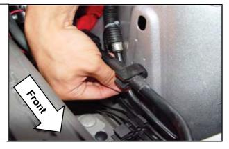
9. Add clean rags under Master Cylinder in order to keep fluid from spilling on vehicle. Unscrew front brake line (Right-closest to driver)
