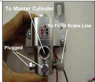
4. Ensure that the new brake line routing is understood prior to installation. However, DO NOT attach lines to solenoid at this time.
