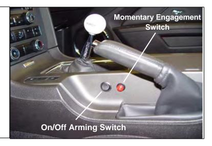
22. Reconnect battery and turn ignition switch to the "ON" position. While still in park and NOT depressing your brake pedal, activate and engage your Hurst Roll/Control system (make sure you can hear the clicking of the solenoid) several times and check fuse. If fuse is burned, check all electrical connections for a short and correct any problems immediately.
