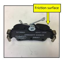
2. Install the pads into the anchor. Put the pad into rotor pathway of the anchor and gently slide the pad and abutments into the inboard side of the anchor. You will be compressing the spring on the side of the abutment as you slide the pad into place. This is a tight fit. Once complete you can do the same for the outboard pad.
