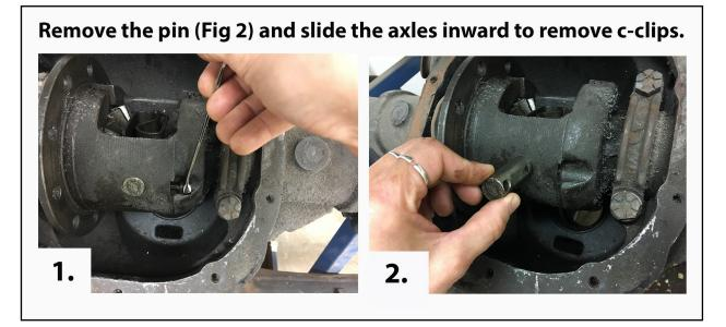
Remove the axles, taking care not to damage the seals. This is a good time to inspect the seals, axles and bearings, replacing as necessary.
