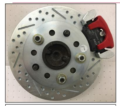
8. View of caliper and rotor installed. Driver side shown. (Left side). Install the hose to the caliper using the supplied banjo bolt and crush washers. Use 1 crush washer on each side of the banjo bolt. Make sure the hose doesn't interfere with any suspension components or the tire/wheel. Torque the banjo bolt to 15 ft lbs.
