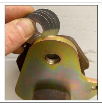
**3.** Put (4) of the supplied 5/8" shims between the top of the bracket and the top of the rear end. This will allow the bracket to sit flat against the rear end. Install the supplied 5/8" hex bolt and nut. **Torque this nut to 145ft lbs.**
