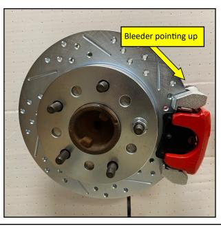
**7.** Install the correct side caliper making sure the bleeder is pointing up.
