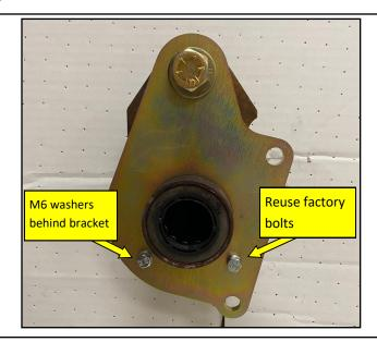
2. Install the Bracket onto the outboard side of the rear end housing. <u>Put a single M6 washer between the bracket and rear</u> <u>end of the 2 lower bolts</u>. This will allow the bracket to sit flat against the rear end. You will reuse your factory bolts for the 2 lower holes. **Torque these to the manufacturers spec.**
