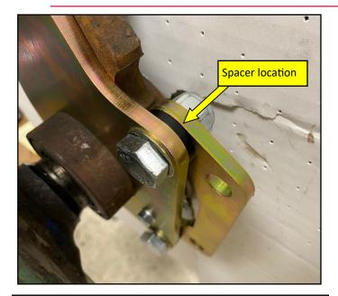
**5.** Next install the intermediate bracket to the inboard side of the base bracket. Use the supplied 12mm hex bolts, washers, spacers and nylock nuts. The spacer goes in between the base bracket and the intermediate bracket. **Torque these nuts to 85ft lbs.**
