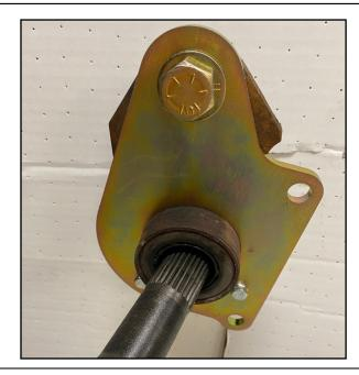
Install the axle back into the rear end and install the clip and rear end pin. Repeat this process for the passenger side.
