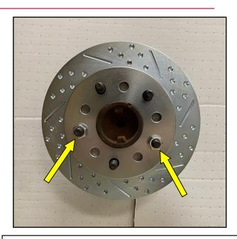
**6.** Install the correct side rotor. (Driver side shown) Make sure to clean off the axle rotor register to make sure the rotor is sitting flat against the axle flange. Secure the rotor with 2 lug nuts and washers.
