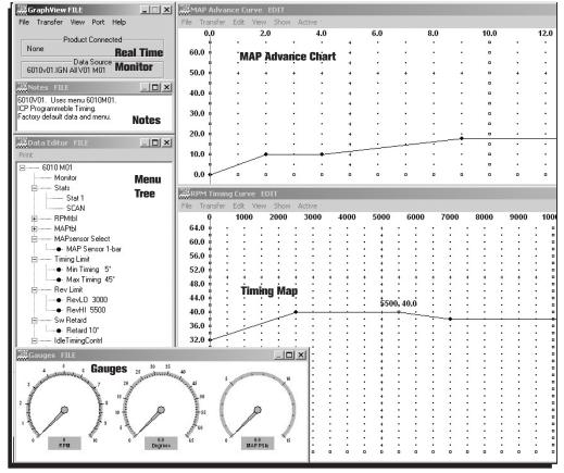
Figure 2 Pro-Data + Screen and Programming Windows.
