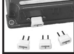
Figure 3 Timing Curve Modules.
