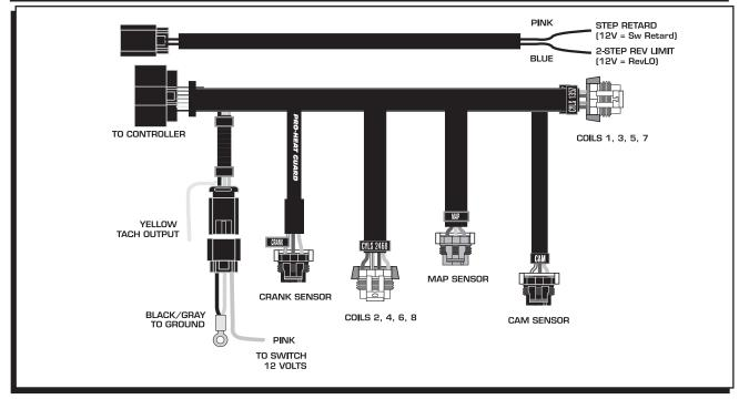
Figure 1 Wiring the MSD Gen III Controller.
