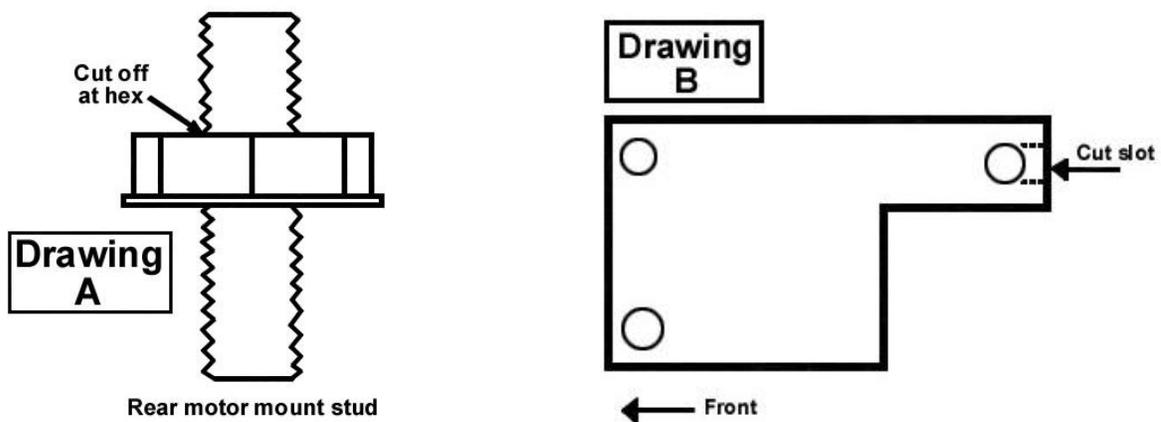
15. After the mount has been modified, insert it back into the engine bay. Do not mount at this time.
