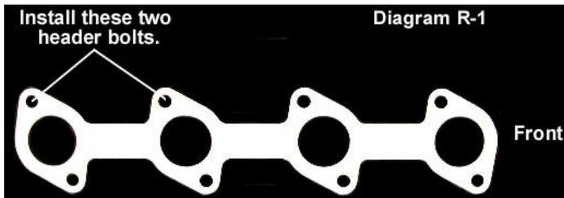
**NOTE:** Some header flange bolt holes are slotted for the ease of bolt installation and are not intended to be installed before the header is inserted into the engine bay. Only the bolts specified in the installation procedure should be installed before the header is inserted into the engine bay.
