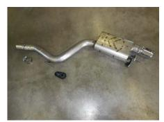
1) Place the new Flowmaster muffler units next to the factory units and swap the front and rear hanger mounts from the stock mufflers to the Flowmaster assemblies. Also, place a provided 2.50" clamp onto the inlet of each assembly. Tighten the clamp just enough to hold in place. **Note:** The protective plastic wrap has been left on the mufflers to protect their finish, please remove prior to starting the vehicle.
