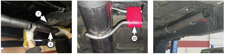
8. Place (x2) **clamps (8)** onto both ends of **muffler (4)** then connect it to extension pipe. Tighten front clamp enough to allow for adjustment.
