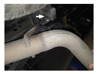
Remove bolts and nuts (x4 ea.) from inlet pipe flanges. Then remove bolts (x2) and wire hanger mount to disassemble exhaust system from vehicle. Retain all bolts and nuts for later use.
