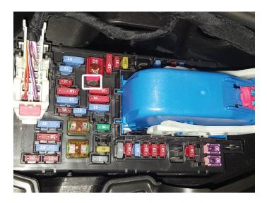
21. Connect female quick disconnect end of controller kit to fuse box.
