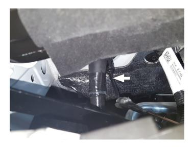
18. Fasten controller kit to a point up and away from interfering with passengers feet.
