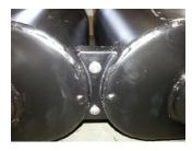
19) Once both mufflers are in place and supported, there are small brackets at the rear that will connect them together. Use the two supplied button electrical connectors to the actuators on the new mufflers.
