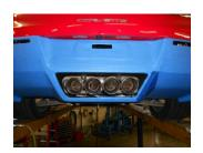
1) Before you begin, please understand that the installation of this system requires significant disassembly. The entire lower rear bumper fascia (Blue portion in photo) must be removed. Because this is a painted body panel, you may want to consider covering it with masking tape for the disassembly/assembly process to prevent any scratches. Note: Do dot turn the vehicle ignition on anytime during the removal/assembly process
