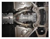
7) Just forward of the rear sub-frame and axles you will find a clamp connection on each of the pipes. Loosen the nut on each of these clamps. Up at the top on each of the pipes that run over the axle, there is an electrical butterfly actuator. Disconnect the electrical connectors.
