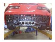
This is what things should look like now. Now you need to start working under the car so either put the car on a hoist, or put the rear of the car on jack stands or ramps. At the rear, between the two factory mufflers you will find that they are connected by small brackets that are secured with small hex bolts. Remove these so that the mufflers can be removed separately.
