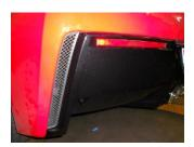
On outside ends of each side of the bumper fascia there are small, plastic vertical grates that must be removed. These are held in place by small clips. Use a small screwdriver to carefully pop these out. At the bottom, where the red and black panels touch, they clip together. Use a small flat blade screwdriver to carefully separate them.
