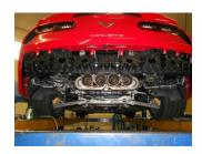
18) Once the actuators have been installed onto the muffler assemblies, the system can be reinstalled on the vehicle. Position one muffler at a time, up over the axle into the clamped connection. Re-use the original bolts to secure the rear hanger bracket up to the frame.
