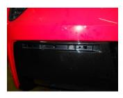
4) On each side of the bumper fascia there is a thin horizontal red reflector that must be removed. It is held in place with clips. Use a small flat blade screw driver to very carefully pop out these two reflectors. Once the reflectors are removed, you will see two hex bolts that secure the fascia to the bumper frame. Remove these two bolts along with two that are located under where the license plate was mounted.
