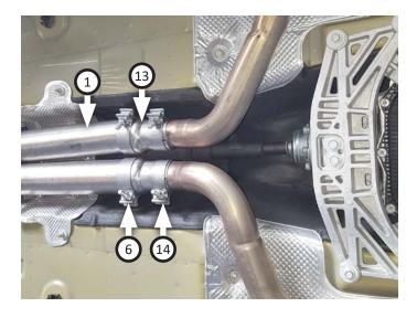
13. Place (x2) clamps (5) onto scavenger pipe (1) inlets then connect it to head pipes withoffset outlet pipe oriented to passenger side). Level and center assembly in drive line tunnel then tighten clamps enough to hold parts.
