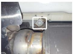
4. Slide front wire hangers out of isolators, loosen clamps behind catalytic converters then carefully remove exhaust system completely from vehicle.
