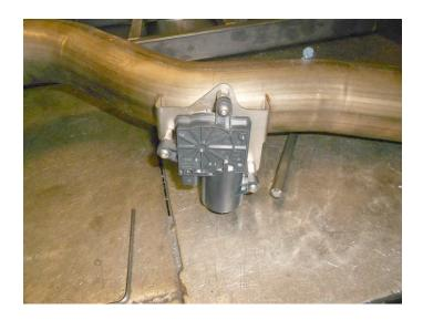
11. Locate (x2) factory exhaust mounts, just forward of rear differential: Remove bolts securing hanger, lift it slightly to clear locating slot and rotate it 180°. Lower hanger back into locating slot and reinstall bolt securely.
