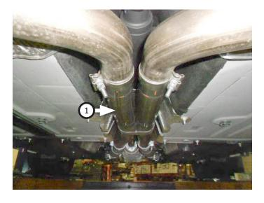
12. Place (x2) clamps (6) onto both muffler (4) inlets then connect them to scavenger pipe, sliding them 1¾" deep. Level mufflers and tighten clamps just enough to hold parts but still allow for adjustment.
