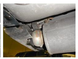
4. Remove (x3) nuts securing actuator to mounts then remove actuator and spring from mount on each tailpipe.
