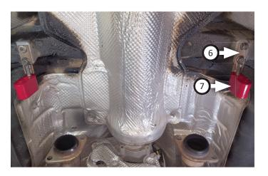
8. Connect left (1) and right (2) resonators onto inlets, inserting wire hangers into isolators. Secure flanges with (x2 ea.) bolts (9), flat washers (11), spacers (10) springs and nuts (removed step 4).
