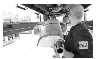
5. Disengage muffler rods from rubber isolaters (3 places), and remove muffler and pipe assembly from vehicle. Remove and retain 2 flange gaskets. Return the spare tire to its stowed position.
