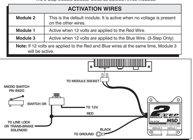
Figure 1 Basic Two Step Module Selector Installation.
