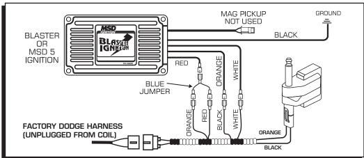
Figure 4 Installation with an MSD 5 or Blaster Ignition.
