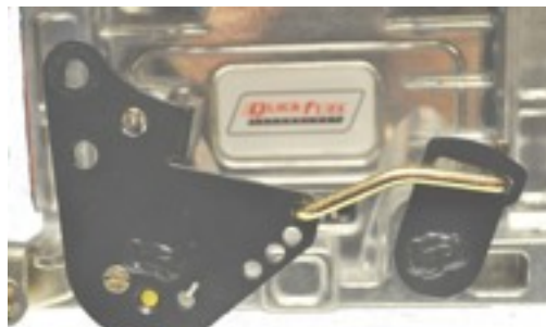
Full Progressive Black Rod - Hole #1 50% Primary Throttle Opening
