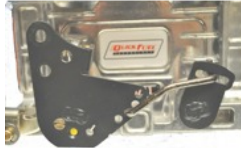
Moderate Progressive Black Rod - Hole #3 25% Primary Throttle Opening
