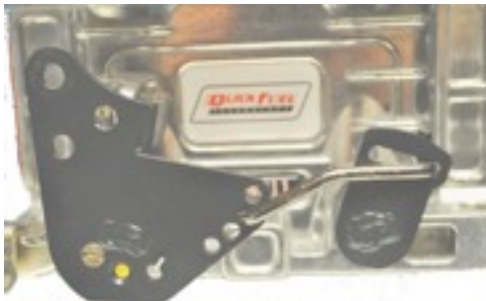
Medium Progressive Black Rod - Hole #2 40% Primary Throttle Opening
