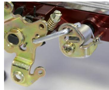
1 to 1 Silver Link, 3 rd Hole, Top Slot
