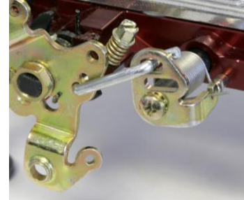
1 to 1 Silver Link, 3 rd Hole, Top Slot
