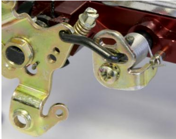
Super Progressive Black Link Top Hole, lower slot 60% primary before secondary opens
