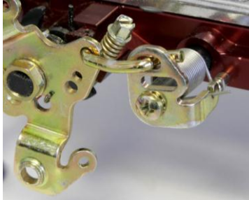
Medium Progressive Gold Link, Top Hole, Top Slot 40% primary before secondary opens This the standard linkage position for most applications.
