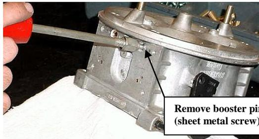
Remove booster pin with dent puller
