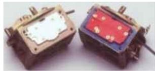
3. When the metering plate is removed, it will be necessary to remove all gasket material from the main body and fuel bowl. Use of a quality carburetor cleaner will help to soften the material making the removal process much easier.
