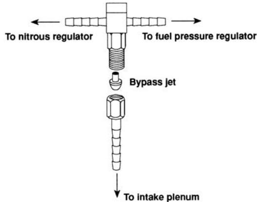
3. Measure and cut a length of vacuum hose (17) to run from one pressure TEE port to the fuel pressure regulator.
