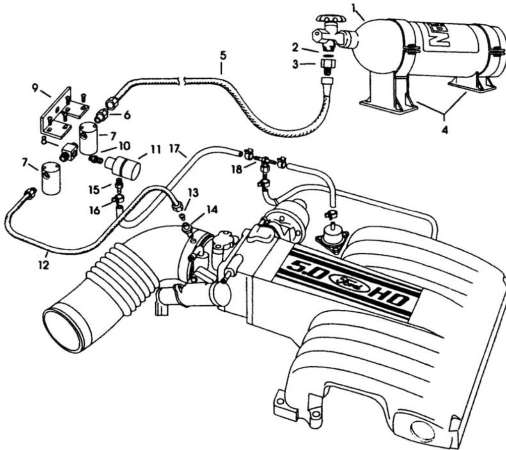
1. Install the bottle nut adapter (3) and washer (2) on the nitrous bottle (1), and tighten securely.
