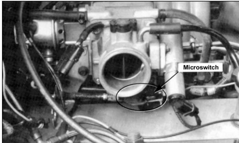
4. Adjust the microswitch to trigger at wide-open throttle. by adjusting the microswitch's position to ensure the actuation arm of the microswitch "clicks" at the same point your throttle linkage reaches WOT against the throttle stop (Position A).
